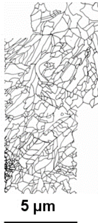
Fig. 68. Microstructure of subgrains inside each ferritic-martensite block (TEM picture: B. Fournier). TEM observations of free dislocations inside blocks [6]. Measurement of subgrain size ( 0.37 \pm 0.1 \mu\text{m} ) and free dislocation density ( 1.1\text{--}1.6 \times 10^{14} \text{ m}^{-2} ) [7]. As-received state.
