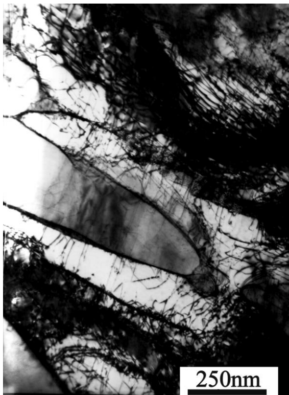
Fig. 68. Microstructure of subgrains inside each ferritic-martensite block (TEM picture: B. Fournier). TEM observations of free dislocations inside blocks [6]. Measurement of subgrain size ( 0.37 \pm 0.1 \mu\text{m} ) and free dislocation density ( 1.1\text{--}1.6 \times 10^{14} \text{ m}^{-2} ) [7]. As-received state.
