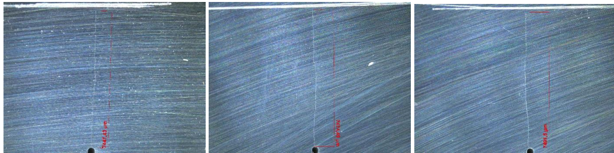
Fig. 3.4.2 The value of crack size after pre-cracking is 7.5 mm.
